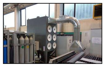
The dust compact filter with horizontal cartridges down flow, automatic cleaning by backwashing with compressed air with electro soundproofed centrifugal fan.
