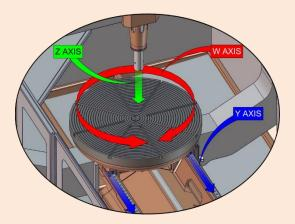
**BLIND SAMPLES.** . Programming properly the limit switches, the tool can enter in blind parts and machining grooves or keyways.
