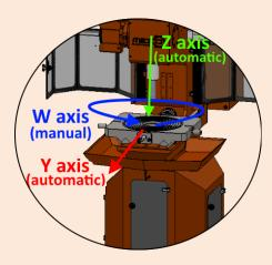
2 AUTOMATIC AXES AND 1 MANUAL. Thanks to the electronic control systems of last generation that have been incorporated in this model for two of its three axes, has achieved greater precision and a higher degree of automation. The machine can work in automatic mode, so that the operator can simply handle replace the part once the machine has finished the process of preprogrammed machining. Undoubtedly, the MECO Keyseaters are designed to increase the production capacity of our customers.
