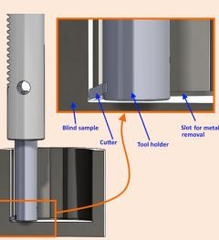
BLIND SAMPLES. . Disassembly the guide bar and programing properly the limit switches, the tool can enter in blind parts and machining grooves or keyways.
