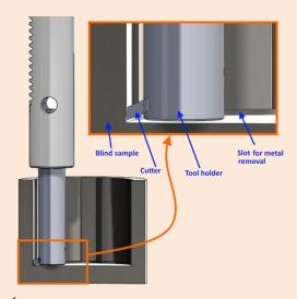
BLIND SAMPLES. . Disassembly the guide bar and programing properly the limit switches, the tool can enter in blind parts and machining grooves or keyways.
