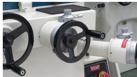
Micro 0.00005" down-feed and cross-feed devices, for 616 model.
