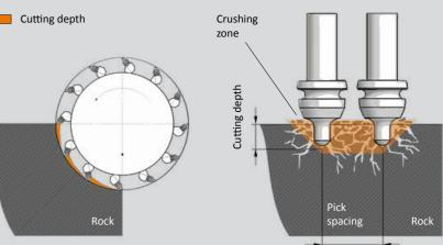
The experience gained from many years of cutting rock has gone into the design of the cutter wheels, drums and chains. They are designed to give maximum cutting performance with minimum wear costs. The selection of picks and boxes, as well as the design of the pick pattern, are part of our continuous product improvement.
