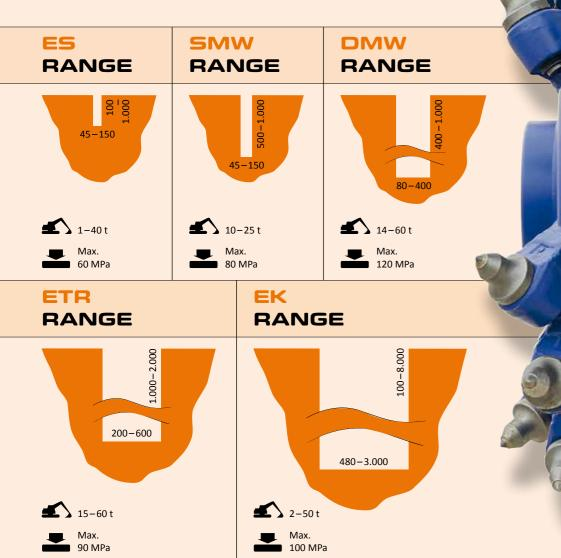
When grinding with round attack picks, each tool penetrates into the rock along parallel paths and breaks material out from the space between the paths. The cutting rate depends to a large degree on the uniaxial compressive strength of the rock being cut. Other significant factors affecting production rates include the hydraulic pressure and flow that the excavator is able to supply to the attachment, as well as the stability and weight of the excavator.
