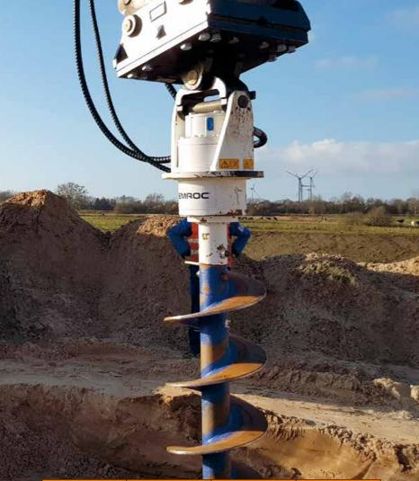
The EBA range of auger drive units allows you to quickly convert your excavator, backhoe or skid-steer loader into a drill rig by simply changing the attachment.
