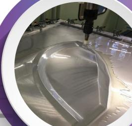
The main use for incremental sheet forming technology is the production of prototypes and short series of sheet metal parts.
